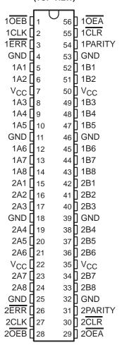
The error (1ERR or 2ERR) output is configured as an open-collector output. The B-to-A parity error flag is clocked into 1ERR or 2ERR on the low-to-high transition of the clock (1CLK or 2CLK) input. 1ERR or 2ERR is cleared (set high) by taking the clear (1CLR or 2CLR) input low.
