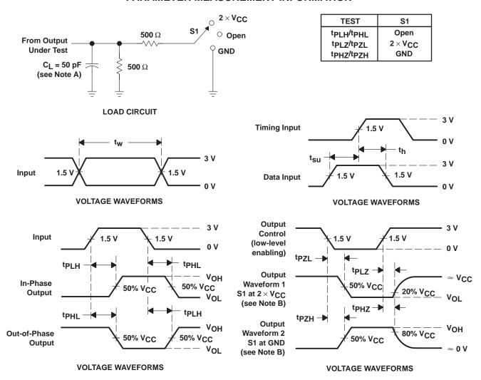
NOTES: A. C<sub>I</sub> includes probe and jig capacitance.
