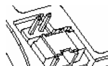
Figure 9: Master Setting for Vertical iDiskOnChip 40-Pin Connector
