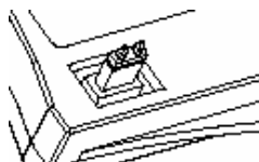
Figure 6: Slave Setting for Vertical iDiskOnChip 44-Pin Connector
