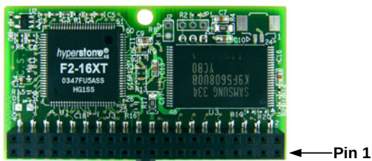
Figure 4: iDiskOnChip Horizontal Version 40 pin, Right-Oriented
