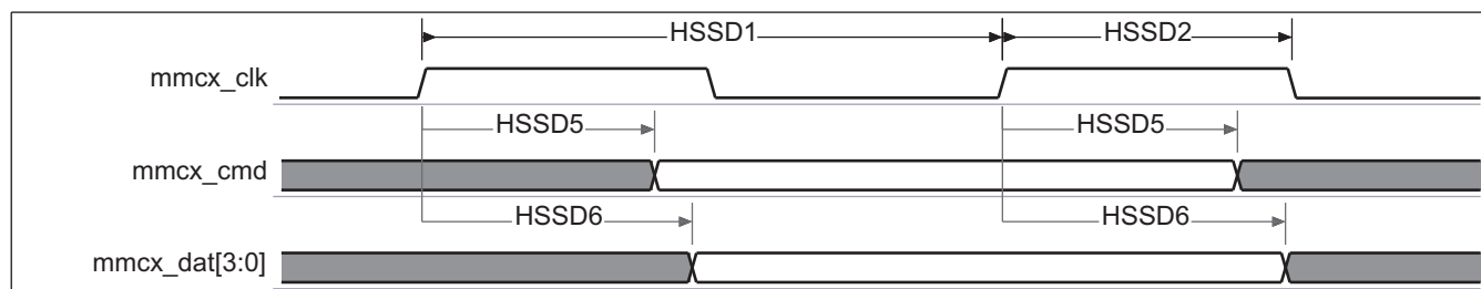
Figure 6-66. MMC/SD/SDIO – High-Speed SD Mode – Data/Command Transmit
