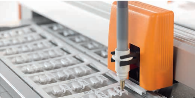
If you use an MCP plotter, even small quantities can be printed.
