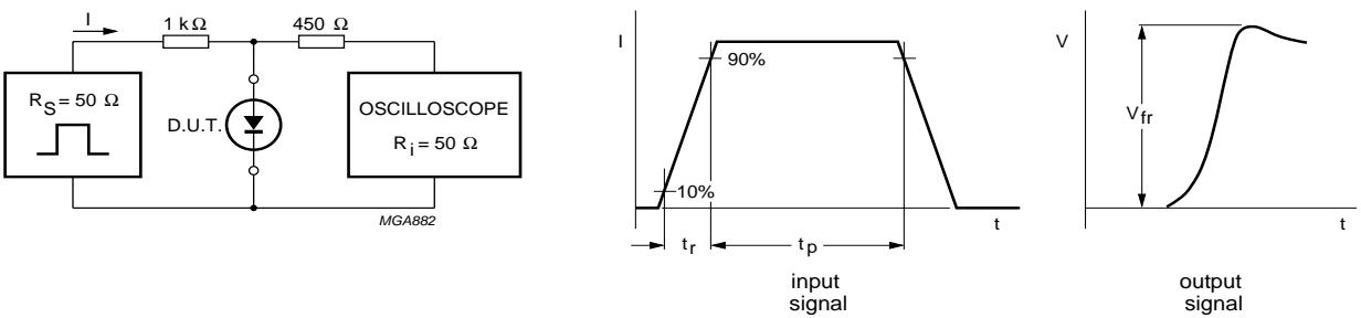
Fig.8 Forward recovery voltage test circuit and waveforms.
