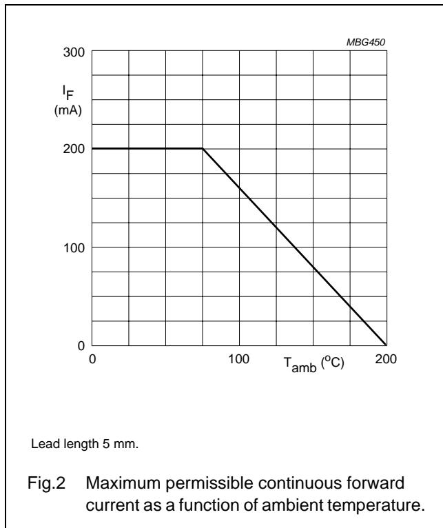
Fig.2 Maximum permissible continuous forward current as a function of ambient temperature.
