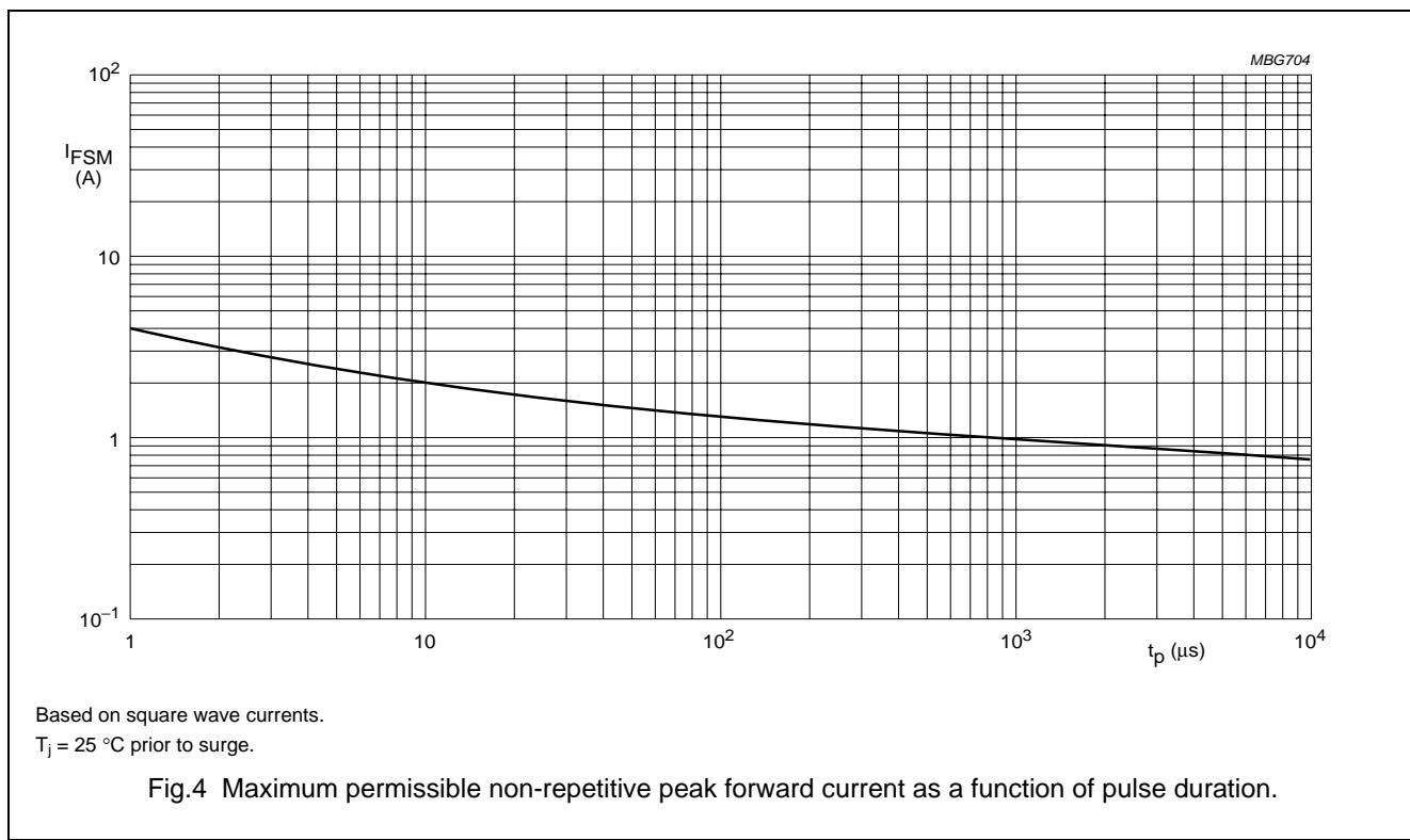
Fig.4 Maximum permissible non-repetitive peak forward current as a function of pulse duration.
