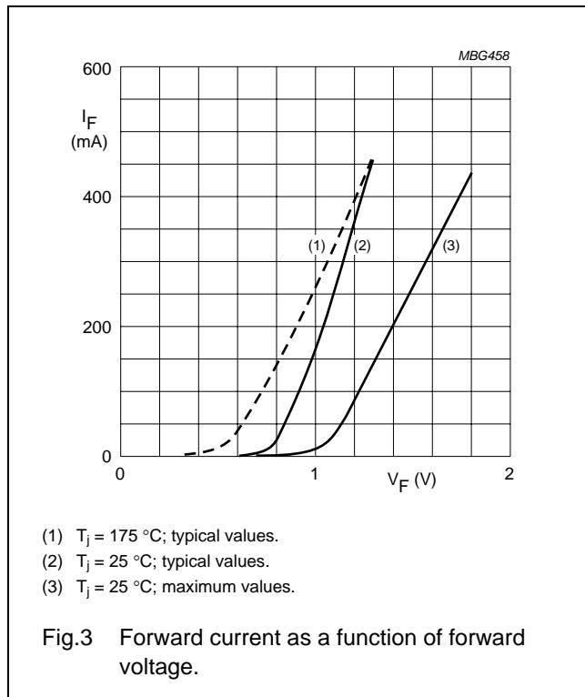
Fig.3 Forward current as a function of forward voltage.
