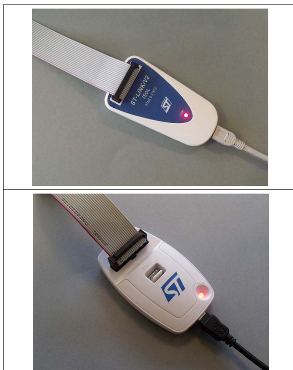
1. The first figure at the top shows the ST-LINK/V2-ISOL, while the second figure shows the ST-LINK/V2.
