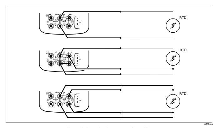
Figure 15. Measuring Temperature with an RTD
