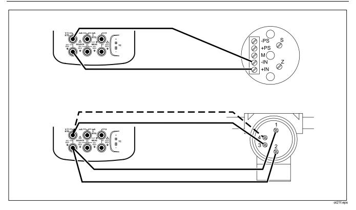
Figure 21. Connections for Simulating an RTD
