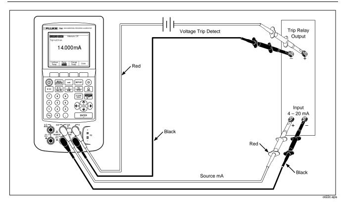
Figure 22. Checking a Relay Output Trip Alarm
