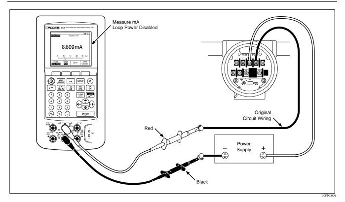
Figure 29. Measuring the Output Current of a Transmitter
