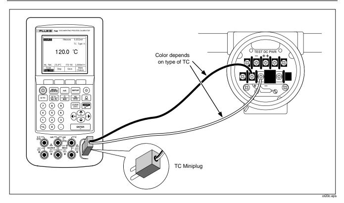
Figure 20. Connections for Simulating a Thermocouple
