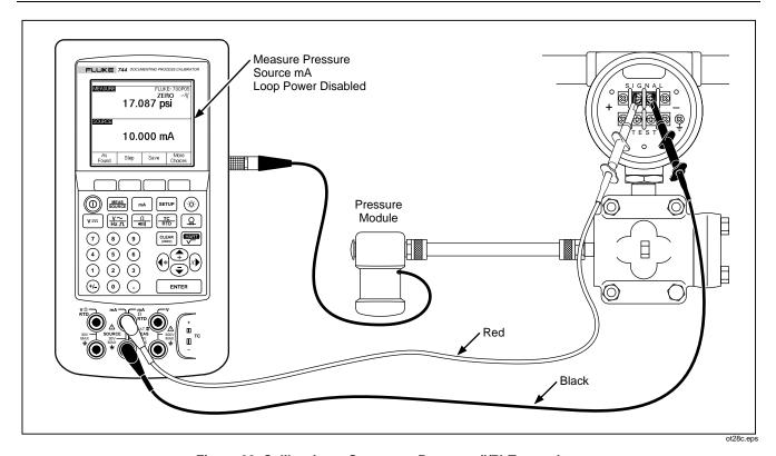
Figure 28. Calibrating a Current-to-Pressure (I/P) Transmitter
