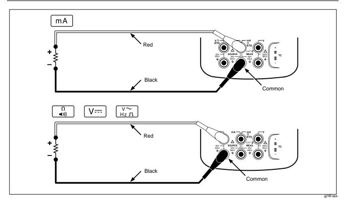
**Figure 16. Electrical Sourcing Connections**
