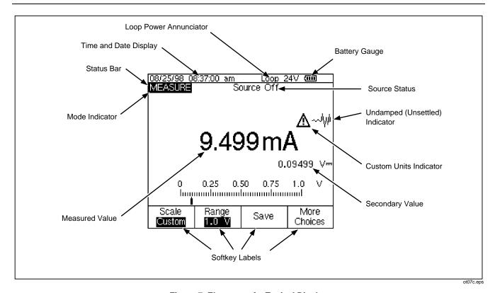
Figure 7. Elements of a Typical Display
