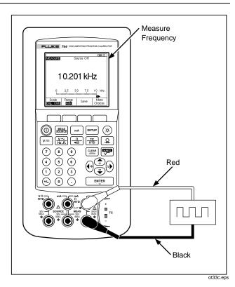
Figure 33. Checking a Tachometer
