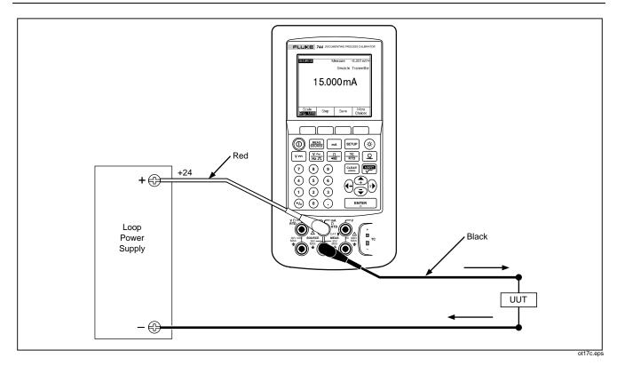
Figure 17. Connections for Simulating a 4 to 20 mA Transmitter
