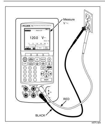
Figure 27. Monitoring AC Line Voltage and Frequency
