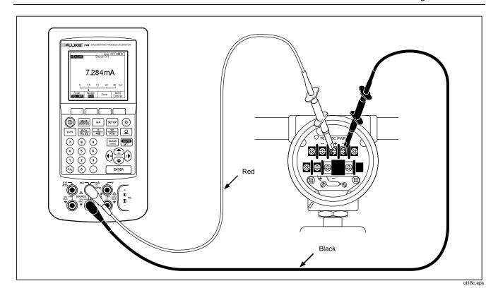
Figure 18. Connections for Supplying Loop Power
