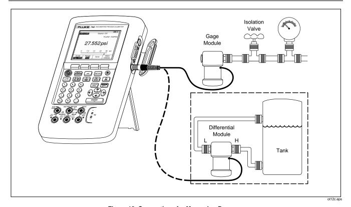
Figure 12. Connections for Measuring Pressure
