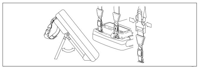
Figure 8. Using the Bail and Installing the Strap
