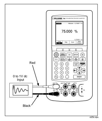
Figure 25. Calibrating a Chart Recorder
