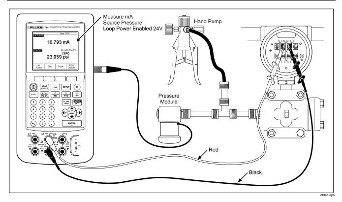
Figure 34. Calibrating a Pressure-to-Current (P/I) Transmitter
