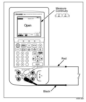
Figure 32. Checking a Switch
