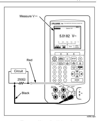
Figure 26. Measuring Voltage Drop
