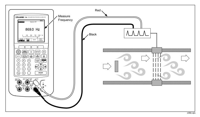
Figure 36. Checking a Vortex Shedding Flowmeter
