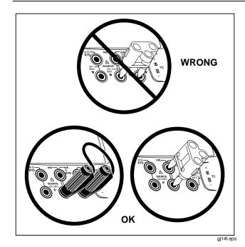
Figure 14. Using a Jumper Correctly
