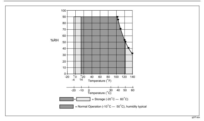
Figure 37. LCD Operating Environment Specification
