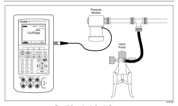
Figure 19. Connections for Sourcing Pressure
