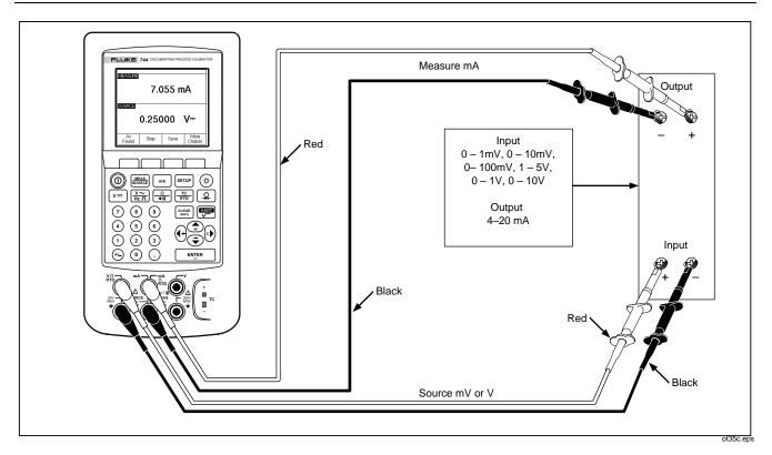
Figure 35. Calibrating a mV to Current Transmitter
