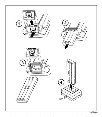
Figure 9. Removing the Battery and Using the Charger
