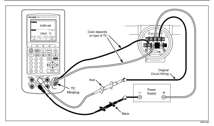
Figure 23. Calibrating a Thermocouple Temperature Transmitter
