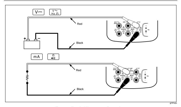
**Figure 10. Electrical Measurement Connections**
