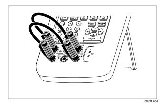
Figure 3. Jumper Connections for Demonstration
