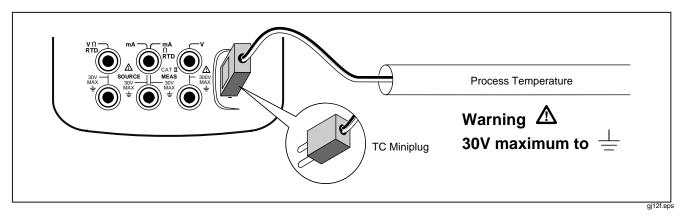
Figure 13. Measuring Temperature with a Thermocouple
