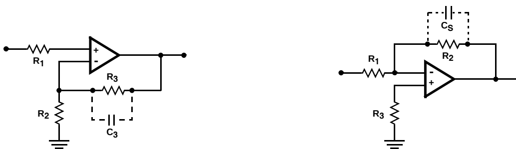
FIGURE 3. SUGGESTED OFFSET VOLTAGE ADJUSTMENT
