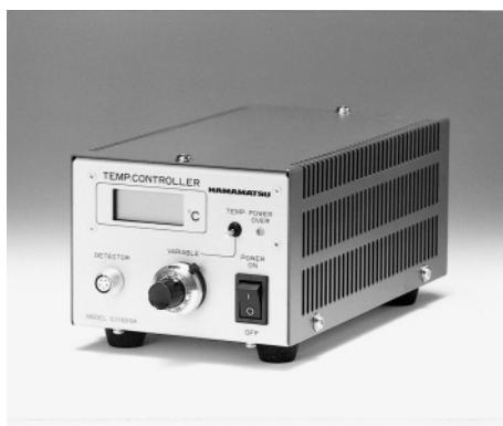
By adjusting the current flowing through the thermoelectric cooler in a one-stage or two-stage thermoelectrically cooled detector, C1103-04 maintains the detector element at a constant temperature. The cooling temperature can be easily set by using the control knob on the front panel.
