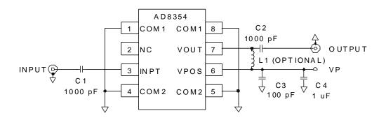
Figure 40. Evaluation Board Schematic
