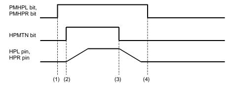
Figure 55. Power-up/Power-down Timing for Headphone-Amp
