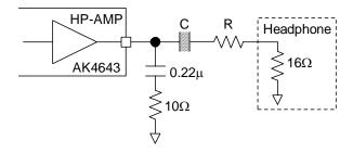
Figure 56. External Circuit Example of Headphone
