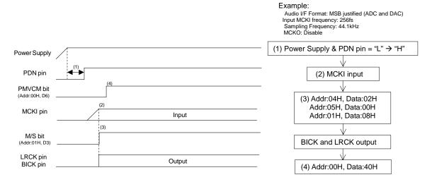
Figure 82. Clock Set Up Sequence (5)
