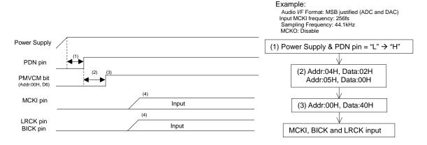
Figure 81. Clock Set Up Sequence (4)
