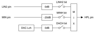
Figure 57. HPL Mixing Circuit (AIN3 bit = "0", HPG bit = "0")
