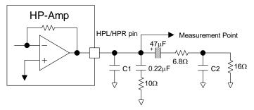
Figure 2. Headphone-Amp output circuit
