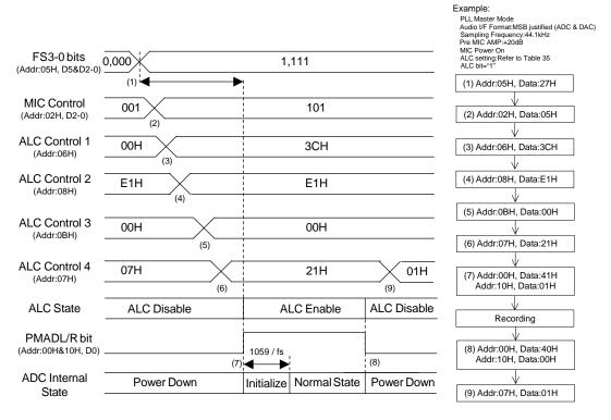
Figure 83. MIC Input Recording Sequence
