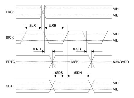
Figure 13. Audio Interface Timing (PLL/EXT Slave mode, Except DSP mode)
