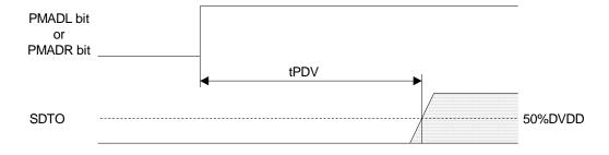
Figure 17. Power Down & Reset Timing 1
