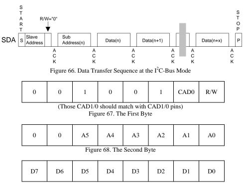
Figure 69. Byte Structure after the second byte
