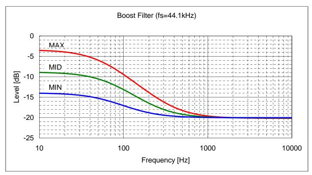
Figure 38. Bass Boost Frequency Response (fs=44.1kHz)
