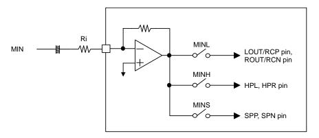
Figure 43 Block Diagram of MIN pin
