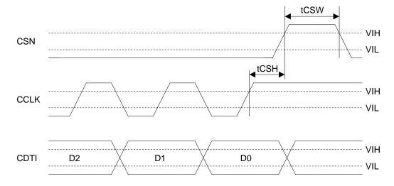
Figure 15. WRITE Data Input Timing
