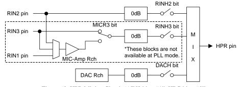
Figure 60. HPR Mixing Circuit (AIN3 bit = "1", HPG bit = "0")
