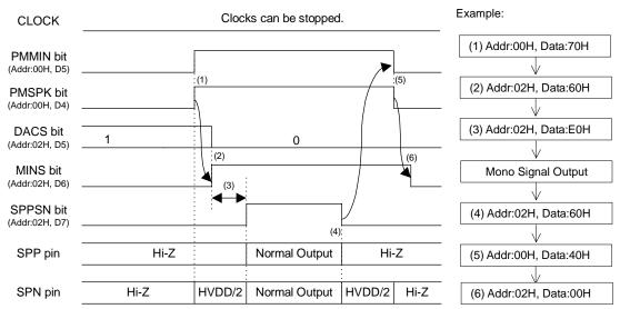
Figure 85. "MIN-Amp → Speaker-Amp" Output Sequence
