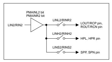
Figure 41. Analog Mixing Circuit (LIN2/RIN2)
