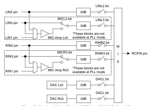
Figure 54. Receiver Mixing Circuit (AIN3 bit = "1", LOVL bit = "0")
