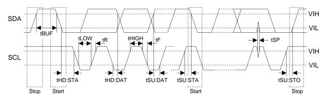
Figure 16. I<sup>2</sup>C Bus Mode Timing
