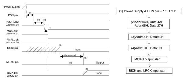
Figure 80. Clock Set Up Sequence (3)
