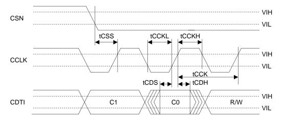
Figure 14. WRITE Command Input Timing
