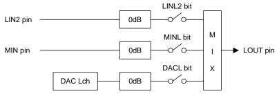
Figure 47. LOUT Mixing Circuit (AIN3 bit = "0", LOVL bit = "0")
