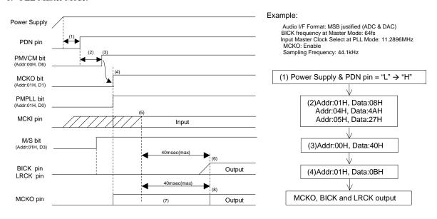
Figure 78. Clock Set Up Sequence (1)
