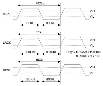
Figure 12. Clock Timing (EXT Slave mode)
