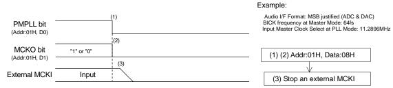
Figure 89. Clock Stopping Sequence (1)
