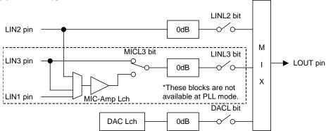
Figure 49. LOUT Mixing Circuit (AIN3 bit = "1", LOVL bit = "0")
