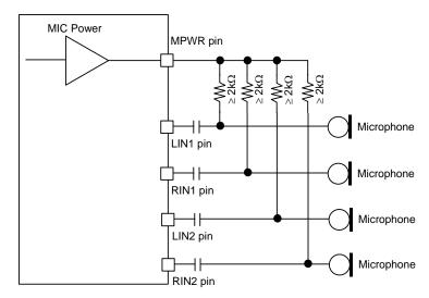
Figure 34. MIC Block Circuit
