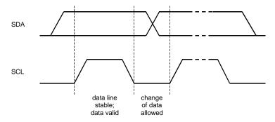
Figure 74. Bit Transfer on the I<sup>2</sup>C-Bus
