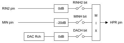
Figure 58. HPR Mixing Circuit (AIN3 bit = "0", HPG bit = "0")
