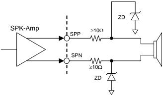
Figure 61. Speaker Output Circuit (Load Capacitance > 30pF)
