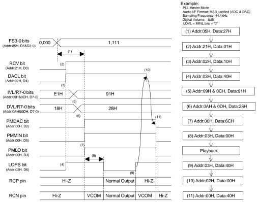
Figure 88. Receiver-Amp Output Sequence
