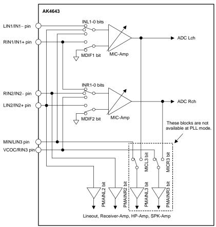
Figure 40. Analog Mixing Circuit
