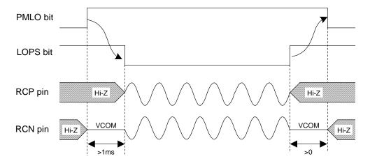
Figure 52. Power-up/Power-down Timing for Receiver-Amp
