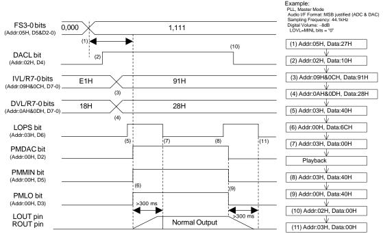
Figure 87. Stereo Lineout Sequence
