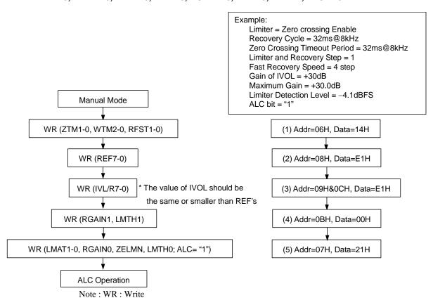
Figure 36. Registers set-up sequence at ALC operation
