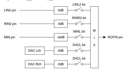
Figure 53. Receiver Mixing Circuit (AIN3 bit = "0", LOVL bit = "0")
