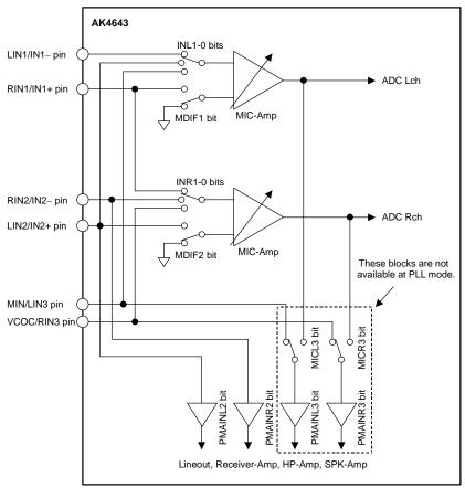
Figure 32. Mic/Line Input Selector
