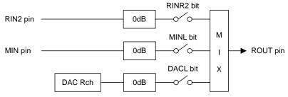
Figure 48. ROUT Mixing Circuit (AIN3 bit = "0", LOVL bit = "0")
