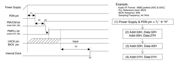
Figure 79. Clock Set Up Sequence (2)
