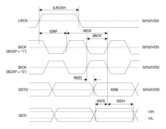
Figure 5. Audio Interface Timing (PLL/EXT Master mode, DSP mode, MSBS = "1")
