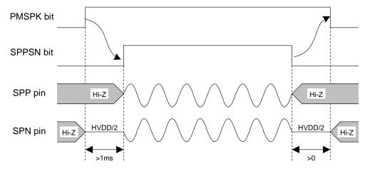
Figure 62. Power-up/Power-down Timing for Speaker-Amp
