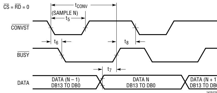
Figure 16. Mode 1a. CONVST Starts a Conversion. Data Outputs Always Enabled
