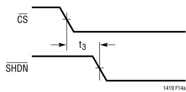
Figure 14a. CS to SHDN Timing
