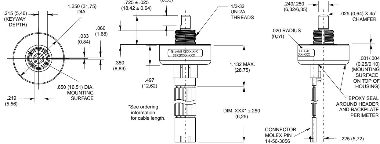
Unless otherwise specified, dimension tolerances are as follows: linear ± .010 (0.25), diameters ± .010 (0.25), angular ± 5°
