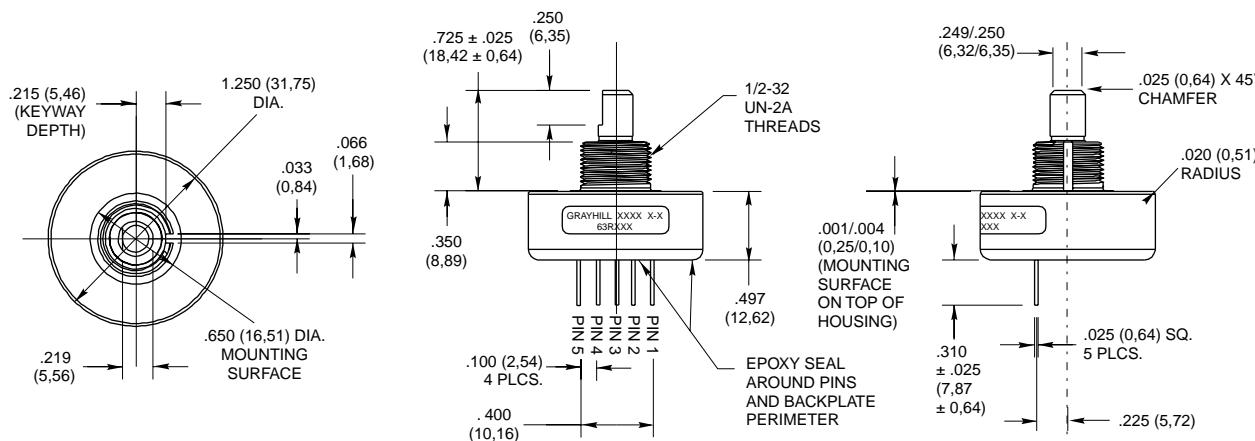
Unless otherwise specified, dimension tolerances are as follows: linear ± .010 (0.25), diameters ± .010 (0.25), angular ± 5°
