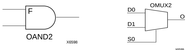
Figure 20: AND & MUX Symbols in XC4000X IOB
