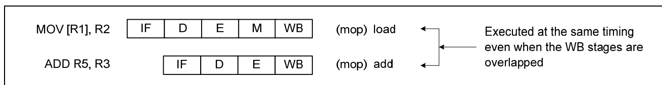
Figure 2.25 When WB Stages for the Memory Load and for the Operation are Overlapped
