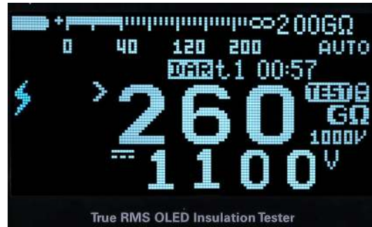
Figure 5. Adjustable insulation test voltage up to 1.1 kV
