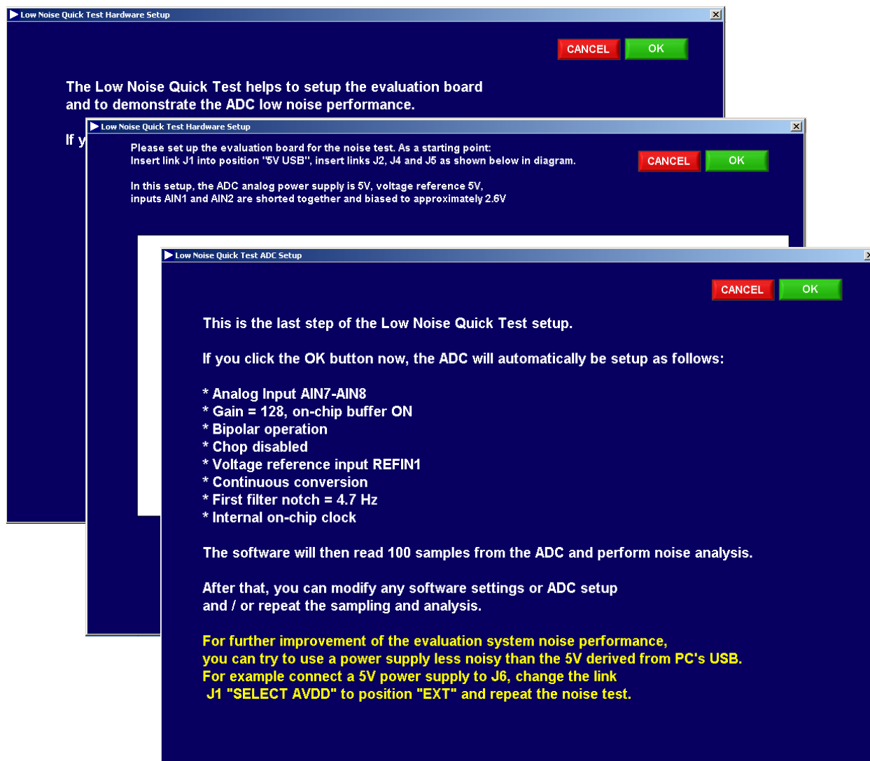
Figure 10. Low Noise Quick Test Hardware Setup
