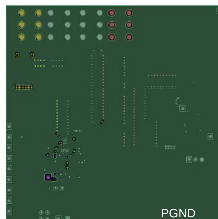
Figure 42c: IRDC3447 Demo board Layout Considerations – Mid Layer 1
