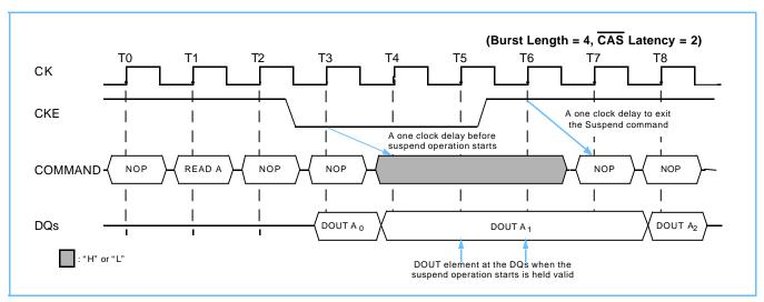
If Clock Suspend mode is initiated during a burst write operation, the input data is masked and is ignored until the Clock Suspend mode is exited.
