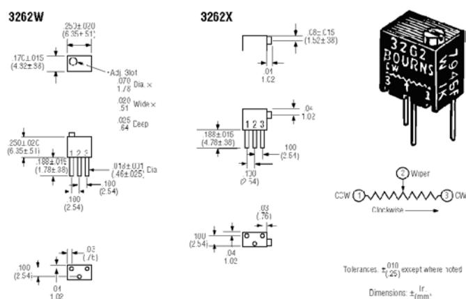
Infinite resolution cermet element. Double chevron shaft seal; plasma etched body. Temperature Range: -65°C to +150°C. Temperature Coefficient: ±100 ppm/°C. Power: 0.5 watt at +85°C. Resistance Tolerance: ±10%.
