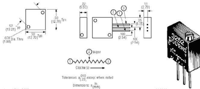
Stable, infinite resolution cermet element. Listed on the DESC QPL for style RJ22 per MIL-R-22097. Low temperature coefficient ±100 ppm/°C over entire temperature and resistance range. High temperature, all plastic case. Superior humidity-proof performance under the most severe conditions. Temperature Range: -65° to +150°C. Power Rating: 0.75 watt at 85°C. Resistance Tolerance: ±10%.
