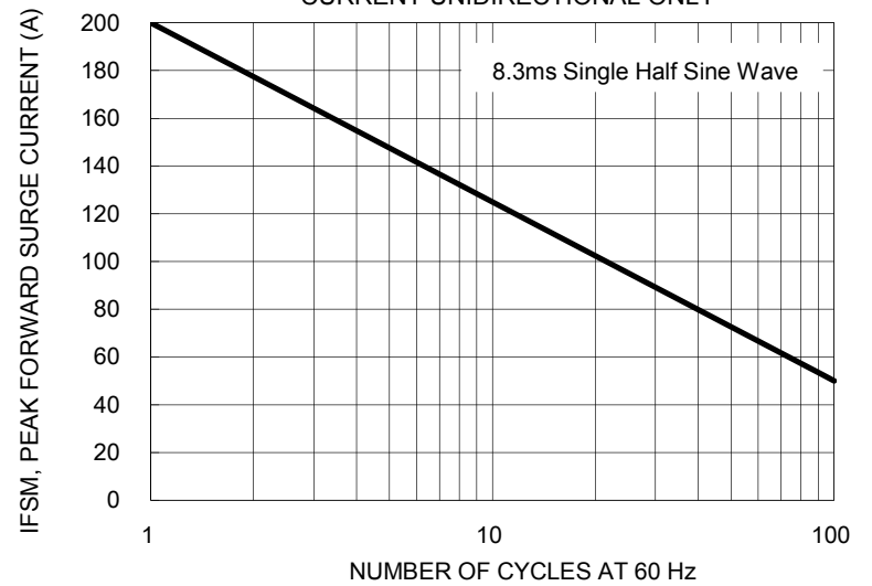
FIG. 4 MAXIMUM NON-REPETITIVE FORWARD SURGE CURRENT UNIDIRECTIONAL ONLY
