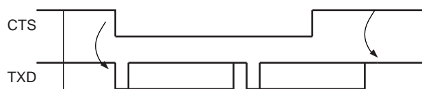
Figure 44-28: Transmitter Behavior when Operating with Hardware Handshaking
