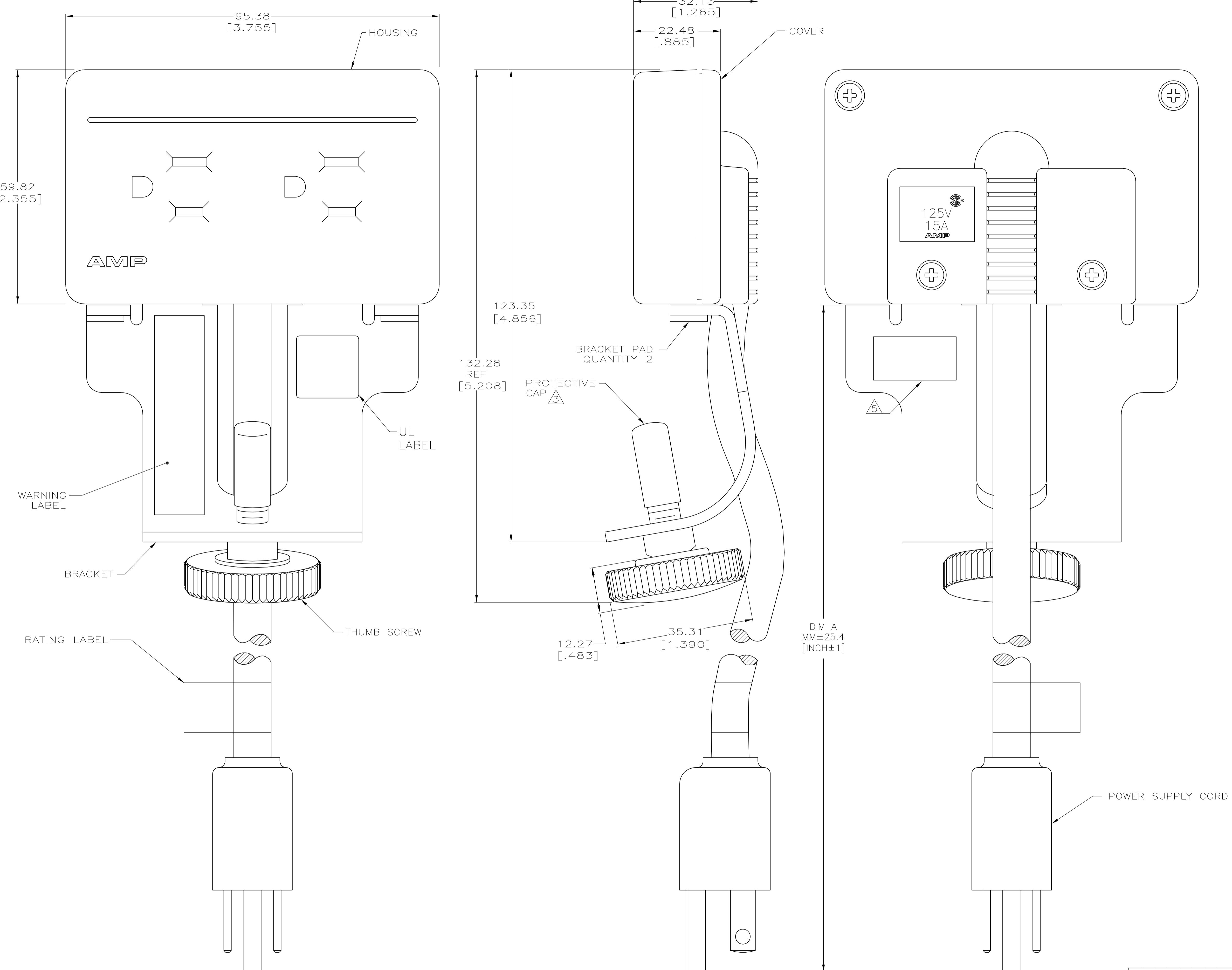
1. MATERIAL: HOUSING AND COVER - POLYCARBONATE MOLDING COMPOUND, 94V-0 RATED. SEE TABLE FOR COLOR.
