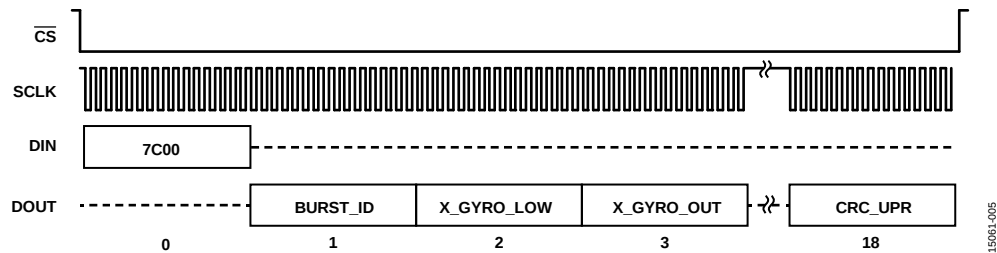
Figure 5. Burst Read Function Sequence Diagram, 19 Segments
