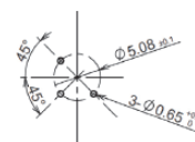
Recommended PCB Pattern Design
