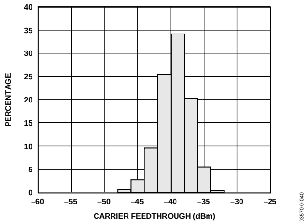
Figure 38. Carrier Feedthrough Distribution at F_{LO} = 1900 MHz ( F_{BB} = 1 MHz, I and Q Inputs Driven in Quadrature at 1.2 V p-p , T_A = 25^\circ\text{C} )
