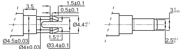
The diagram illustrates the snap-in part of a plastic actuator which can be used to rotate the Series 51 Standalone module.
