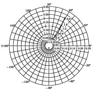
$\begin{array}{l} \text{S}_{22e} \\ \text{V}_{\text{CE}} = 8\text{V} \\ \text{I}_{\text{C}} = 5\text{mA} \\ \text{Ta} = 25^{\circ}\text{C} \\ \text{(UNIT : } \Omega\text{)} \end{array}$
