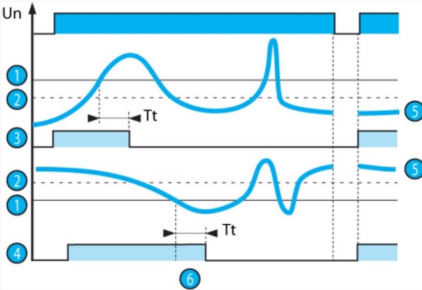
The under or overvoltage threshold value is set by a graduated potentiometer by reading the  $U_n$  scale to be monitored directly.
