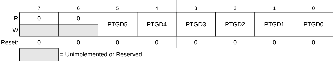
Figure 6-42. Port G Data Register (PTGD)
