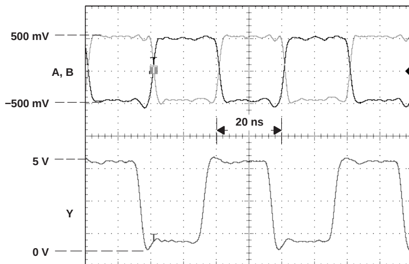
Figure 10. Receiver Inputs and Outputs, 50 Mbps Signaling Rate
