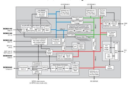
The BCM3214 is a highly integrated CMTS MAC integrated circuit for use in DOCSIS 2.0 and advanced TDMA PHY-layer CMTS products. With hardware support for concatenation parsing, fragment reassembly, payload header suppression, and advanced TDMA physical layer data rates, the BCM3214 serves as the heart of a next-generation CMTS. The BCM3214 provides a powerful, yet cost-effective solution for a variety of CMTS architectures.
