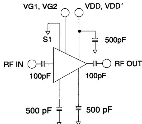
1. Self-bias operation is obtained by connecting +6 volts to both VDD and VDD' pads, grounding pad S1, and connecting pads GND1 and GND2 to separate bypass 500pF MOS capacitors.
