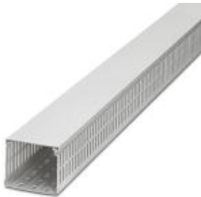
Cable duct, white, comprising upper part and mounting base, width: 30 mm, height: 100 mm, length: 2000 mm
