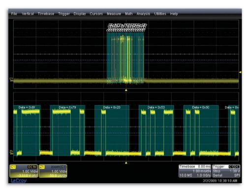
writes to specific sub-address memory blocks in the EEPROM. It can also aid in monitoring DATA outputs from sensors, such as analog-to-digital converters, and triggering when DATA is outside a safe operating range. In both cases, verifying proper operation becomes a simple task.
