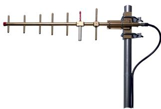
1-port sector (yagi) antenna, 824–896 MHz, 60° HPBW, fixed electrical tilt. Mounting pipe diameter, max. 3".
