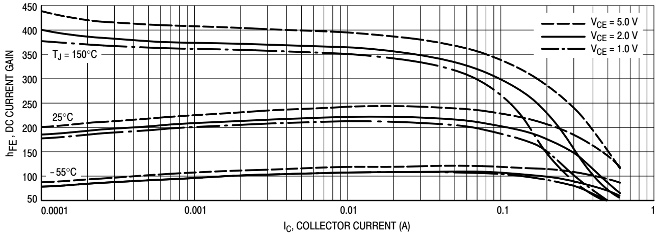
Figure 12. DC Current Gain
