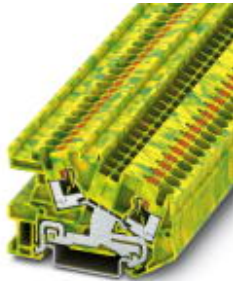
Installation terminal block, Push-in connection, Cross section: 0.2 mm² - 6 mm², AWG: 24 - 10, Width: 6.2 mm, Color: green-yellow, Mounting type: NS 35/7,5, NS 35/15
