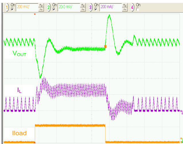
Figure 14. Load Transient 50 to 250mA, 3.6VIN, 5µs/div.
