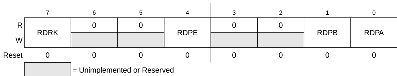
Figure 18-15. Reduced Drive Register (RDRIV)
