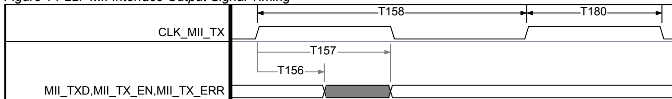
Figure 14-22. MII Interface Output Signal Timing
