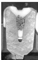
Cross section of wire crimped in the upper tier
