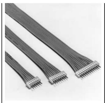
This low-profile, board-in connector, with a mounting height of only 4.25mm (.167") and a thickness of 2.4mm (.094"), is soldered directly onto printed circuit boards. The solder tail of the contact is resilient for easy assembly. The housing lances facilitate insertion of contacts.
