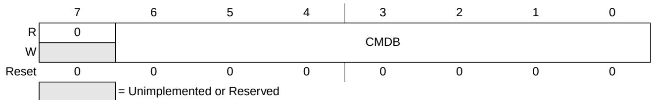
Figure 3-11. Flash Command Register (FCMD - NVM User Mode)
