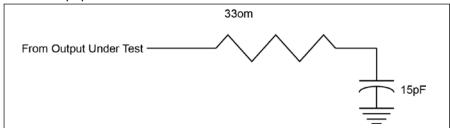
2> Timing Definitions for output clock rise and fall time Measurement
