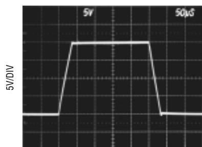
Large-Signal Transient Response
