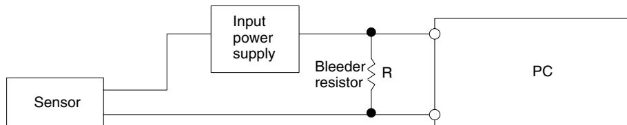
If the leakage current is less than 1.3 mA, there should be no problem. If the leakage current is greater than 1.3 mA, determine the value and rating for the bleeder resistor using the following formulas.
