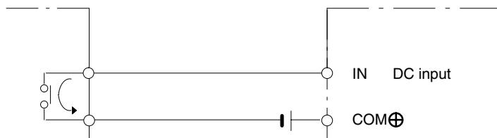
When using the following configurations, the sensor and Input Unit should receive their power from the same supply.
