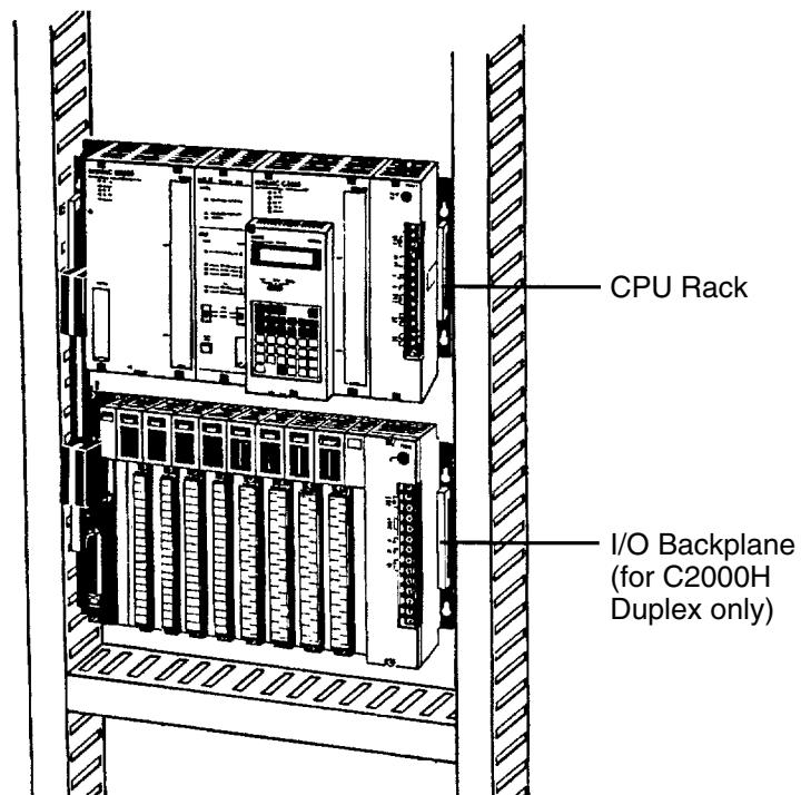
The following figure shows a side view of a mounted CPU and two Expansion I/O Racks. There should be a distance of 70 to 120 mm between the mounted Units.
