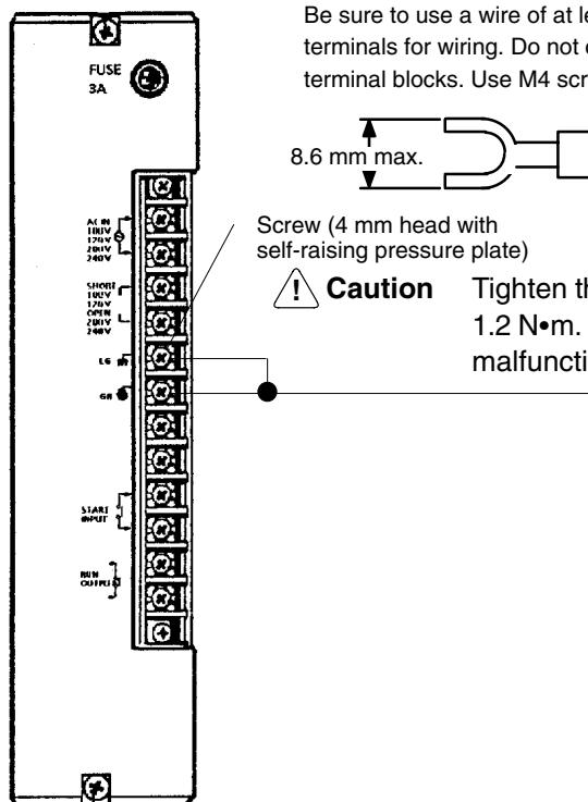
Be sure to use a wire of at least  $1.25 \text{ mm}^2$  in thickness. Use crimp terminals for wiring. Do not connect bare stranded wires directly to terminal blocks. Use M4 screws for tightening crimp terminals.
