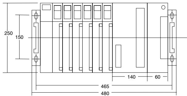
**C2000H Duplex CPU Rack****3G2C5-BC001**
