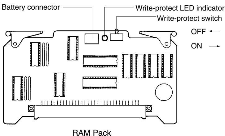
To write data to the RAM Pack, move the write-protect switch to the OFF position. After data is written to the RAM Pack, be sure to move the write-protect switch to the ON position to protect the data from further alterations. If you try to write data to the Memory Pack while the write-protect switch is in the ON position, the message DISABLED ROM will appear on the Programming Console.
