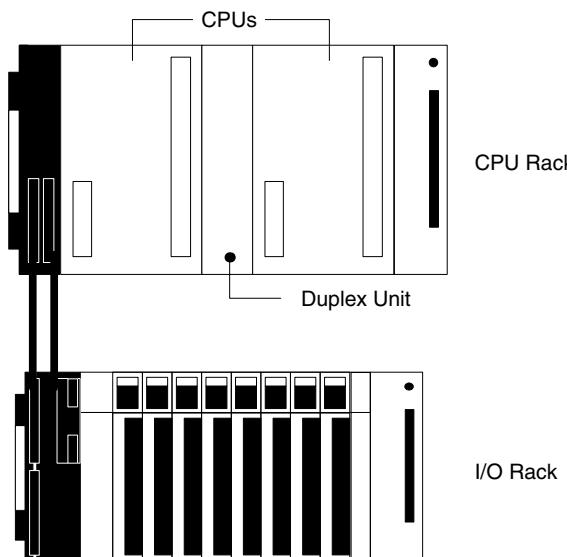
While the Duplex System is in operation, one of the two CPUs has "active" status and the other CPU has "standby" status. The active CPU executes the program and controls the I/O Units while the standby CPU merely executes the program, but does not control the I/O Units. The status of the CPUs can be determined by setting the selector switch on the front panel of the Duplex Unit.
