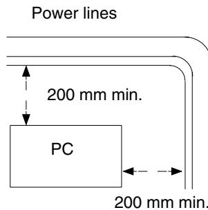
Whenever possible, use wiring conduit to hold the I/O wiring. Standard wiring conduit should be used, and it should be long enough to completely contain the I/O wiring and keep it separated from other cables.
