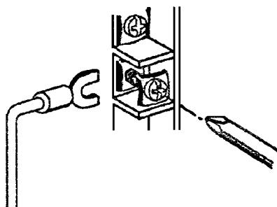
Use ring crimp terminals for wiring. Do not connect bare stranded wires directly to terminal blocks.
