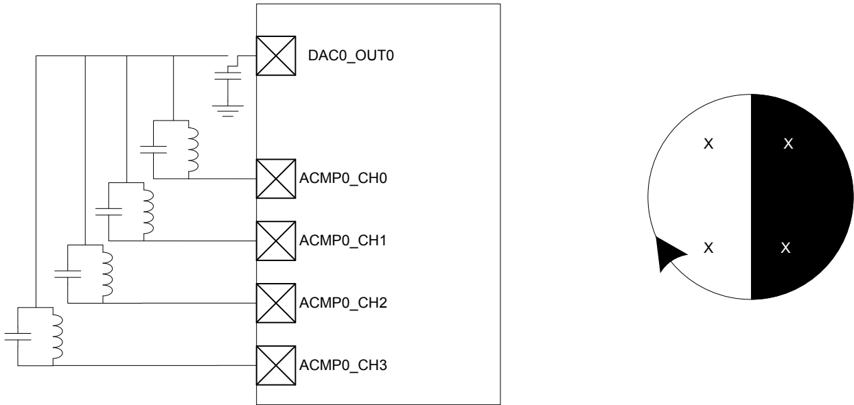
Figure 28.16. LC sensor setup
