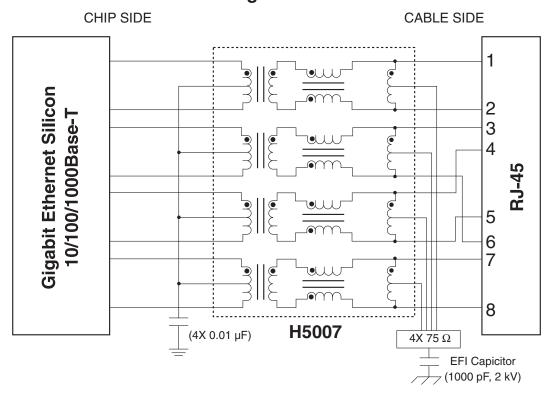
The above circuit is a simple interface for a gigabit transformer connectiong to both the Gigabit Ethernet silicon and the RJ-45 connector.
