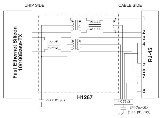
The above circuit is a simple interface for a Fast Ethernet tranformer connecting to both the Fast Ethernet silicon and the RJ-45 connector. In order to design a gigabit application, simply replace the Fast Ethernet Silicon, the Fast Ethernet transformer and the rest of the passive components with a gigabit ethernet silicon, a gigabit transformer and the rest of the passive components.
