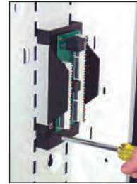
Step 2 - Secure with two screws
